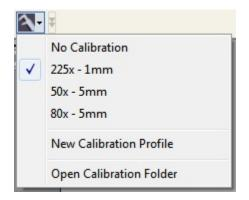
For best results, it is recommended that you select a calibration profile close to the magnification you are using. For example, if the microscope is at 75X magnification and you have calibration profiles setup for 50x, 80x and 200x, it is best to use the profile setup at the closest magnification, which in this case would be 80x.
