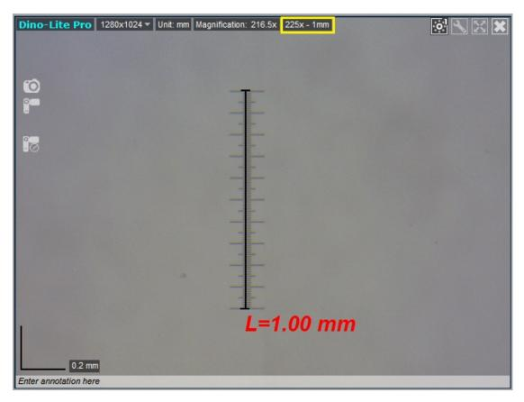
When a calibration profile is in use, a box on the top of the preview window will display your adjusted magnification rate.
