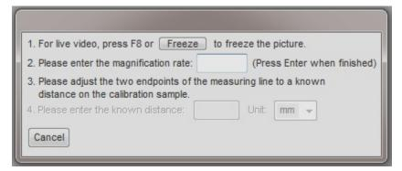
6. Enter the magnification that can be read from the Dino-Lite. Press Enter when finished. In this example I will be calibrating at 225X.
