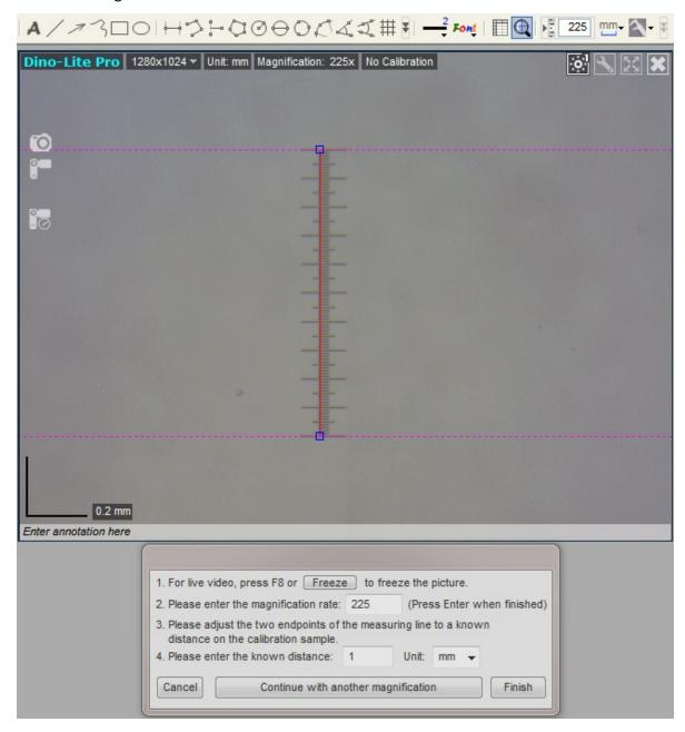
13. Enter the units of measurement by selecting the "Unit" dropdown box.
