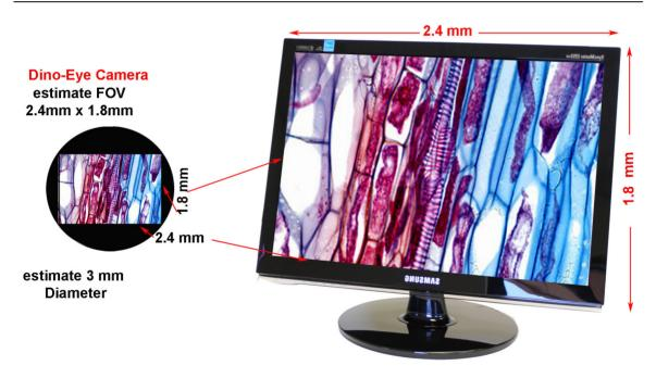
The AM series eyepiece cameras are equivalent to a 20x eyepiece (most traditional eyepiece are using 20x or 16x). Thus for a given objective lens, the eyepiece cameras will usually provide a smaller field of view and larger magnification of the original image when compared to the traditional eyepiece. To achieve a larger field of view with the DinoEye, use a less powerful objective lens, or attach a reducer lens such as a 0.5x lens.
