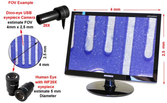
The AM series eyepiece cameras are equivalent to a 20x eyepiece (most traditional eyepiece are using 20x or 10x). Thus for a given objective lens, the eyepiece cameras will usually provide a smaller field of view and larger magnification of the original image when compared to the traditional eyepiece. To achieve a larger field of view with the DinoEye, use a less powerful objective lens, or attach a reducer lens such as a 0.5x lens.
